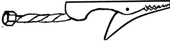
The Tweezers are used in conjunction with the Quantum Clip. After attaching the Quantum Clip to an object or, when the object cannot be gripped by the Clip, pressing the Clip with the closed jaws against an object, to activate the Quantum Clip simply squeeze the points of the Tweezers firmly but gently across any of the two opposing flat surfaces on the hexagon nut of the Clip.
